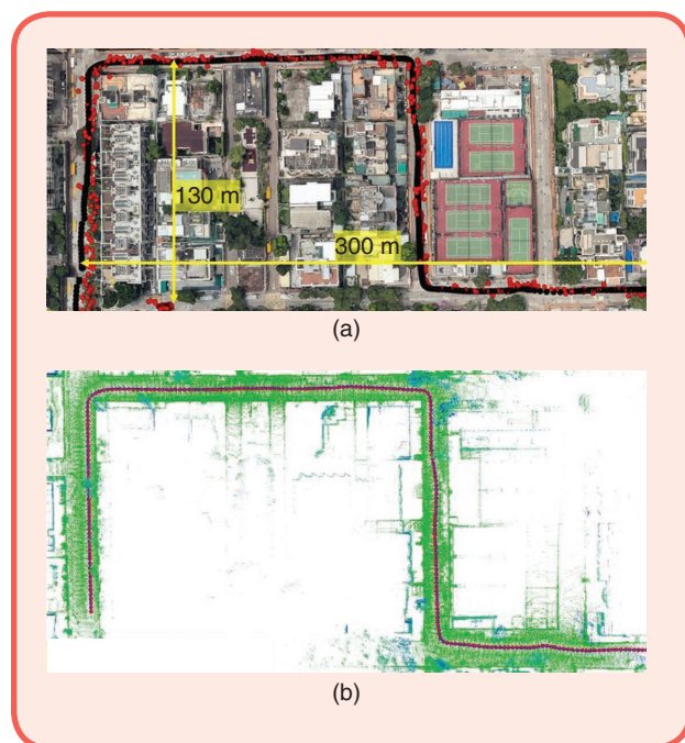
FIG 1 (a) The performance of GNSS stand-alone positioning. The red circles indicate the GNSS-positioning result, and the black circles represent the ground truth. (b) The GNSS–lidar integration, where green points signify the point cloud map and pink circles denote the trajectory generated by the GNSS–lidar integration. The background image of Figure 1(a) is captured from Google Earth.
