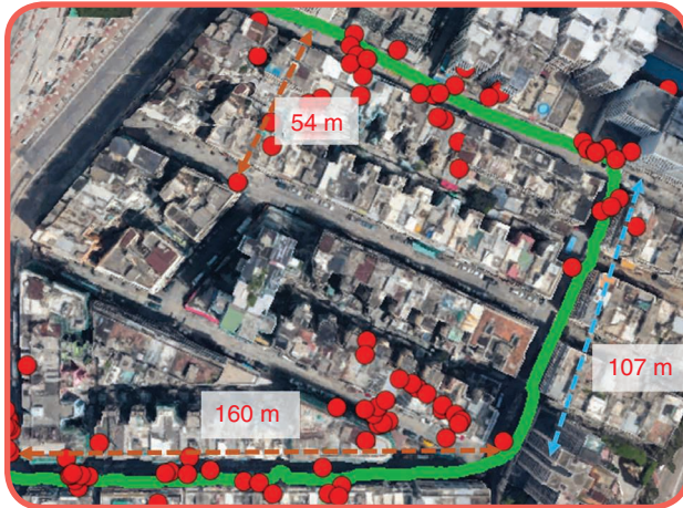
FIG 10 Experiment 1: the trajectory of the autonomous vehicle is indicated by the green curve, and the red circles convey the GNSS-positioning result. The background image of Figure 10 is captured from Google Earth.
